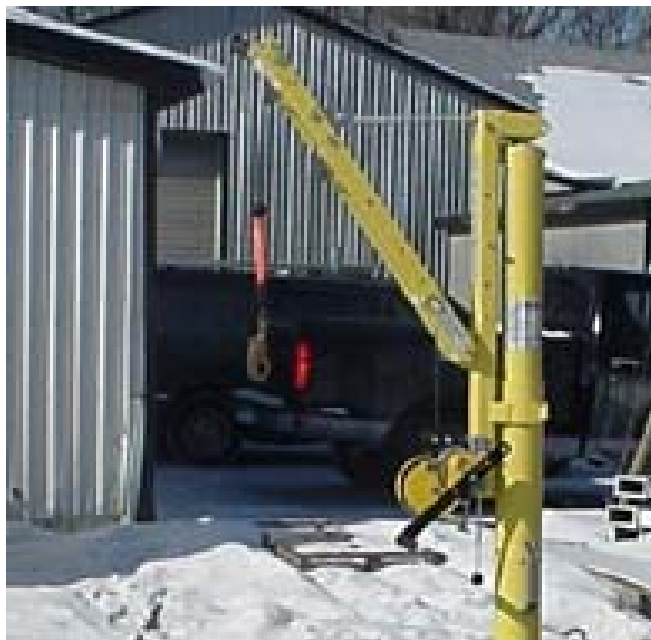
GM193 Boom Kit with single winch mount
