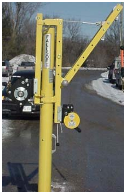
GM193 & 198 Boom Kit with double winch mount
